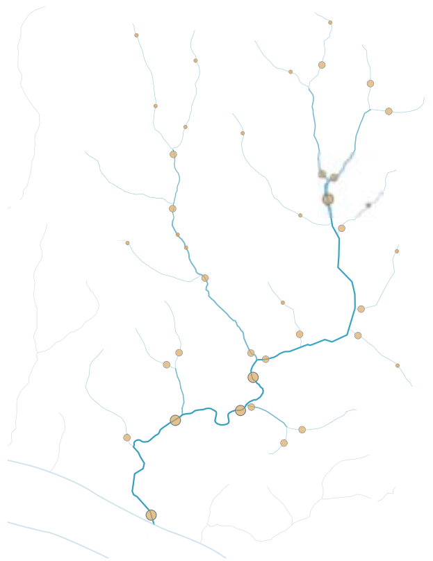
The stream protocol sets testing points based upon stream order and its relationship to land use.
