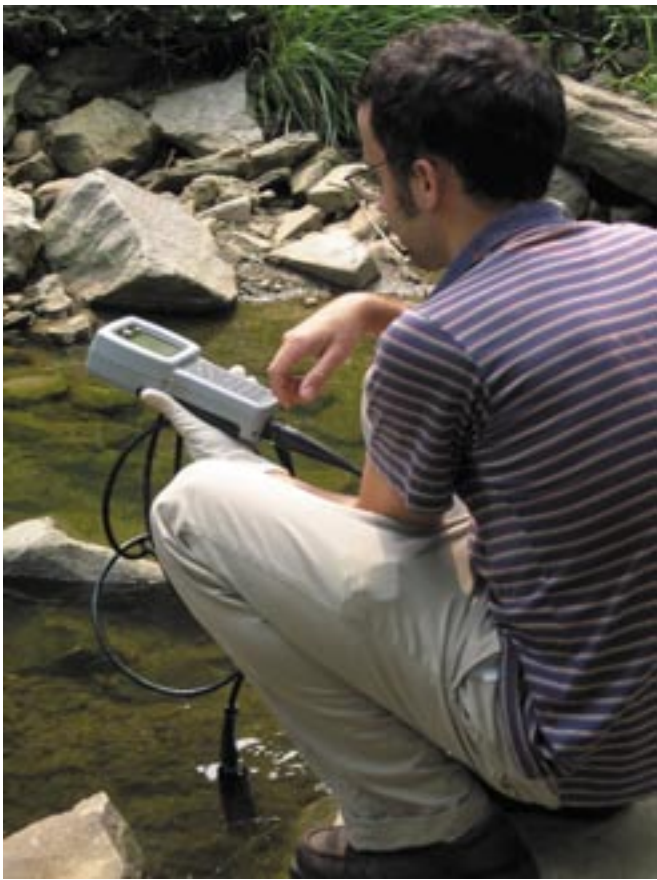
Using the YSI - 556 Meter, provides quick and consistent water quality data, temperature, pH, dissolved oxygen and conductivity.
