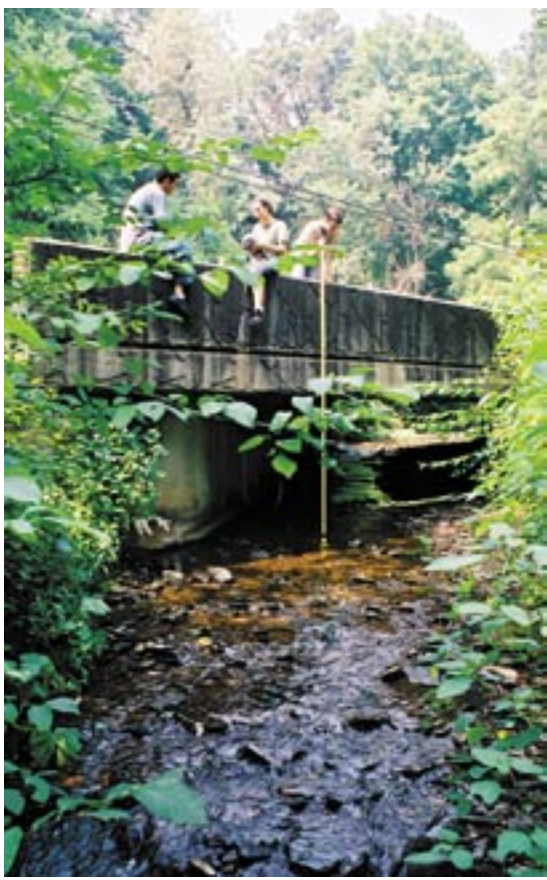
Sampling in the field with the YSI meter and a bridge - sample rod and a GPS unit.
